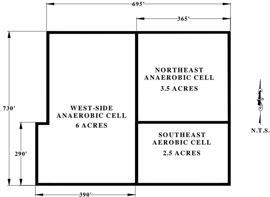
**Detail 1. Overview of Module 6D bioreactor cells**
