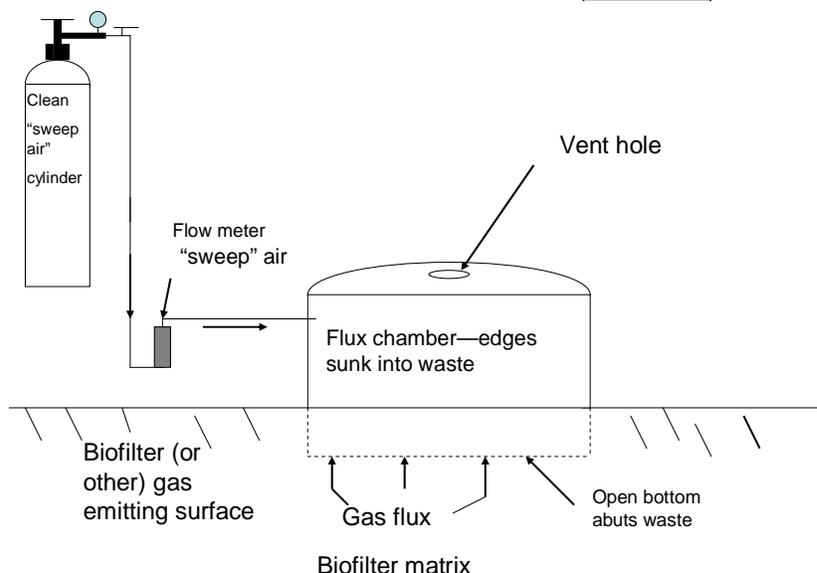
**Figure 4. Flux test setup**
