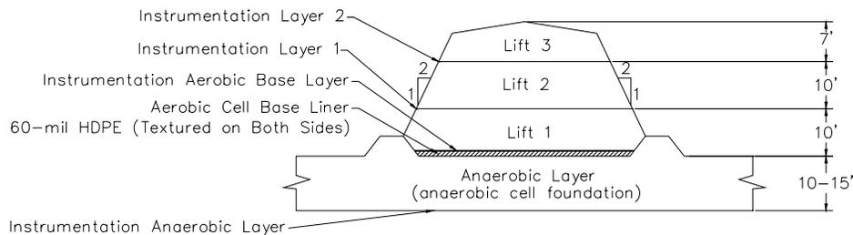
**Detail 7. Cross-section of the Southeast aerobic cell**
