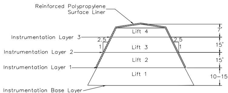
**Detail 6. Northeast anaerobic cell cross-section**
